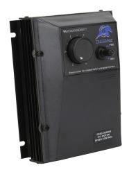
IronHorse GSD5 series DC general purpose drive, 120/240 VAC, 1-phase, 1/8 to 1hp at 90 VDC and 1/4 to 2hp at 180 VDC, 10.8A, NEMA 4/12, wall mount, built-in reverse, potentiometer input, SCR output.
