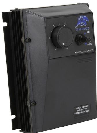
IronHorse GSD5 series DC general purpose drive, 120/240 VAC, 1-phase, 1/8 to 1hp at 90 VDC and 1/4 to 2hp at 180 VDC, 10.8A, NEMA 4/12, wall mount, field-install reverse, current or potentiometer input, SCR output.
