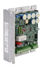
IronHorse GSD4A series DC general purpose drive, 120/240 VAC, 1-phase, 1/8 to 1/2hp at 90 VDC and 1/4 to 2hp at 180 VDC, 6A, open frame, panel mount, field-install reverse, potentiometer input, SCR output.
