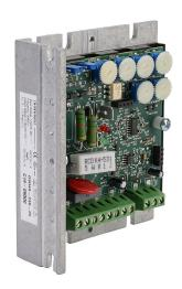
IronHorse GSD4A series DC general purpose drive, 120/240 VAC, 1-phase, 1/50 to 1/8hp at 90 VDC and 1/25 to 1/4hp at 180 VDC, 2A, open frame, panel mount, field-install reverse, potentiometer input, SCR output.
