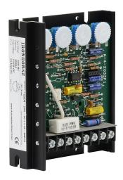
IronHorse GSD4 series DC general purpose drive, 24/36 VAC, 1-phase, 1/50 to 1/6hp at 24-36 VDC, 5.5A, open frame, panel mount, field-install reverse, potentiometer input, SCR output.
