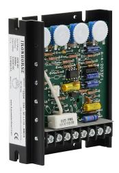
IronHorse GSD4 series DC general purpose drive, 24/36 VAC, 1-phase, 1/50 to 1/6hp at 24-36 VDC, 5.5A, open frame, panel mount, field-install reverse, potentiometer input, SCR output.
