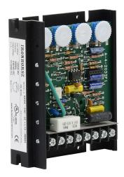
IronHorse GSD4 series DC general purpose drive, 120/240 VAC, 1-phase, 1/8 to 1/2hp at 90 VDC and 1/4 to 1hp at 180 VDC, 5.5A, open frame, panel mount, field-install reverse, potentiometer input, SCR output.
