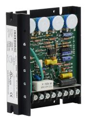
IronHorse GSD4 series DC general purpose drive, 120/240 VAC, 1-phase, 1/50 to 1/8hp at 90 VDC and 1/25 to 1/4hp at 180 VDC, 1.2A, open frame, panel mount, field-install reverse, potentiometer input, SCR output.
