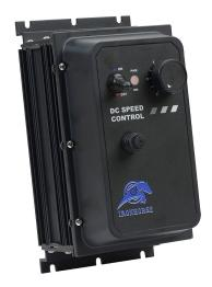
IronHorse GSD4 series DC general purpose drive, 120/240 VAC, 1-phase, 1/8 to 1hp at 90 VDC and 1/4 to 2hp at 180 VDC, 10A, NEMA 4X, wall mount, field-install reverse, potentiometer input, SCR output.
