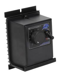
IronHorse GSD3 series DC general purpose drive, 12/24 VAC, 1-phase, 1/50 to 1/25hp at 12 VDC and 1/25 to 1/12hp at 24 VDC, 3A, NEMA 4, wall mount, field-install reverse, potentiometer input, SCR output.
