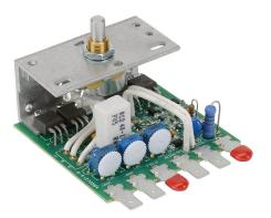
IronHorse GSD3 series DC general purpose drive, 12/24 VAC, 1-phase, 1/50 to 1/40hp at 12 VDC and 1/25 to 1/20hp at 24 VDC, 2A, open frame, J style mount, field-install reverse, potentiometer input, SCR output.
