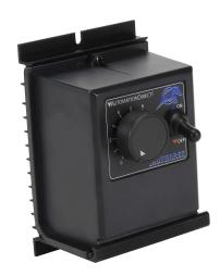
IronHorse GSD3 series DC general purpose drive, 120/240 VAC, 1-phase, 1/50 to 1/3hp at 90 VDC and 1/25 to 2/3hp at 180 VDC, 3A, NEMA 4, panel mount, field-install reverse, potentiometer input, SCR output.
