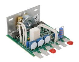
IronHorse GSD3 series DC general purpose drive, 120/240 VAC, 1-phase, 1/50 to 1/6hp at 90 VDC and 1/25 to 1/3hp at 180 VDC, 2A, open frame, L style mount, field-install reverse, potentiometer input, SCR output.
