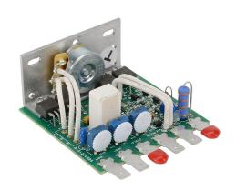
IronHorse GSD3 series DC general purpose drive, 120/240 VAC, 1-phase, 1/50 to 1/6hp at 90 VDC and 1/25 to 1/3hp at 180 VDC, 2A, open frame, L style mount, field-install reverse, potentiometer input, SCR output.
