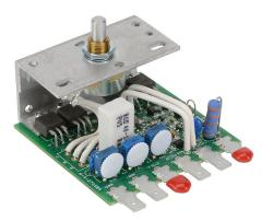
IronHorse GSD3 series DC general purpose drive, 120/240 VAC, 1-phase, 1/50 to 1/6hp at 90 VDC and 1/25 to 1/3hp at 180 VDC, 2A, open frame, J style mount, field-install reverse, potentiometer input, SCR output.
