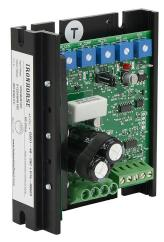
IronHorse GSD1 series DC full-featured drive, 12-48 VDC, 1-phase, 1/50 to 1/4hp at 12 VDC and 1/12 to 1hp at 48 VDC, 20A, open frame, panel mount, field-install reverse, potentiometer input, PWM output.
