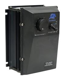
IronHorse GSD1 series DC full-featured drive, 12-48 VDC, 1-phase, 1/50 to 1/8hp at 12 VDC and 1/12 to 1/2hp at 48 VDC, 10A, NEMA 4X, wall mount, field-install reverse, potentiometer input, PWM output.
