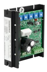
IronHorse GSD1 series DC full-featured drive, 12-48 VDC, 1-phase, 1/50 to 1/8hp at 12 VDC and 1/12 to 1/2hp at 48 VDC, 10A, open frame, panel mount, field-install reverse, potentiometer input, PWM output.
