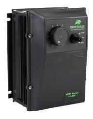
IronHorse GSD1 series DC reversing drive, 12/24 VDC, 1-phase, 1/50hp at 12 VDC and 5/16hp at 24 VDC, 15A, NEMA 4X, wall mount, built-in reverse, potentiometer input, PWM output.
