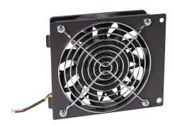
DURApulse GS4 series board cooling fan, replacement, 120 x 120 x 25.4mm, 24 VDC. For use with GS4 E frame drives. Electrical connector included.
