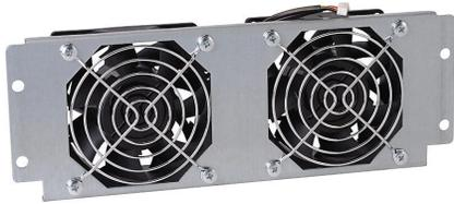
DURApulse GS4 series main cooling fan, replacement, 80 x 80 x 38mm, 24 VDC. For use with GS4 D0 frame drives. Electrical connector included.
