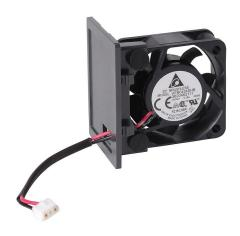
DURApulse GS4 series board cooling fan, replacement,  $40 \times 40 \times 15$ mm, 24 VDC. For use with 230V GS4 C frame drives. Electrical connector included.
