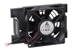
DURApulse GS4 series main cooling fan, replacement,  $80 \times 80 \times 25$ mm, 24 VDC. For use with GS4-27P5 and GS4-4010 B frame drives. Electrical connector included.
