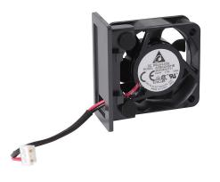
DURApulse GS4 series board cooling fan, replacement, 40 x 40 x 15mm, 24 VDC. For use with GS4 B frame drives. Electrical connector included.
