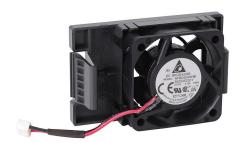
DURApulse GS4 series main cooling fan, replacement,  $40 \times 40 \times 15$ mm, 24 VDC. For use with GS4 A frame drives. Electrical connector included.
