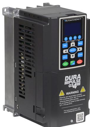
DURApulse GS4 series AC high-performance drive, NEMA 1, 460 VAC, 3hp with 3-phase input, SVC or V/Hz mode, A frame, RS-485, Modbus and BACnet, 100kA SCCR. Optional EtherNet/IP and Modbus TCP cards available.
