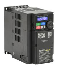
DURApulse GS30 series AC high-performance drive, enclosed, 230 VAC, 3hp with 1-phase input, SVC, V/Hz, FOC, encoder or torque mode, C1 frame, RS-485, integrated dynamic braking. Optional communication, encoder and I/O modules available.
