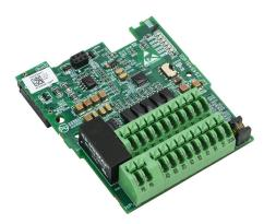
DURApulse GS30 series encoder module, line driver (differential) encoder input. For use with GS30 series AC drives. Supports 1-phase and 2-phase input and output.
