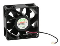
DURApulse GS30 series main cooling fan, replacement, 204 x 87 x 50mm, 24 VDC. For use with GS30 series G frame AC drives. Electrical connector included.
