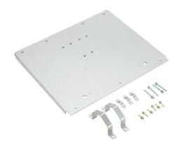
DURApulse GS30 series EMC shield plate, for use with GS30 series I frame AC drives. Allows motor lead shields to be grounded at the drive.
