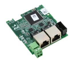
DURApulse GS30 series communication module, EtherCAT CoE protocol, 2 ports, (2) Ethernet (RJ45) port(s). For use with GS30 series AC drives.
