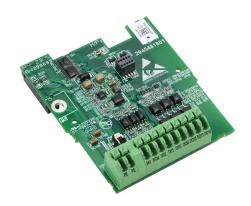
DURApulse GS30 series discrete combo module, Input: 3-point, 24 VDC, sinking/sourcing selectable, Output: 3-point, 48 VDC, sinking/sourcing selectable, 30 mA/point, 50 mA resistive output current. For use with GS30 series AC drives.
