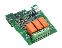
DURApulse GS30 series relay output module, 3-point, 250 VAC/30 VDC, (3) Form B (SPDT) relays, 2 isolated common(s), 1 point(s) per common. Screw terminal blocks included.
