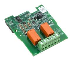
DURApulse GS30 series relay output module, 2-point, 240 VAC/30 VDC, (2) Form C (SPST) relays, 2 isolated common(s), 1 point(s) per common. Screw terminal blocks included.
