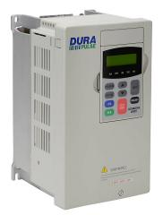
DURApulse GS3 series AC general purpose drive, enclosed, 460 VAC, 5hp with 3-phase input, SVC or V/Hz mode, B frame, RS-485, integrated dynamic braking.
