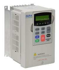
DURApulse GS3 series AC general purpose drive, enclosed, 460 VAC, 3hp with 3-phase input, SVC or V/Hz mode, A1 frame, RS-485, integrated dynamic braking.
