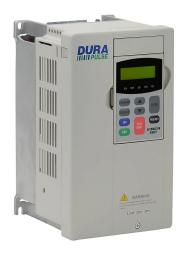
DURApulse GS3 series AC general purpose drive, enclosed, 230 VAC, 3hp with 3-phase and 1-phase input, SVC or V/Hz mode, B frame, RS-485, integrated dynamic braking.
