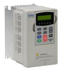
DURApulse GS3 series AC general purpose drive, enclosed, 230 VAC, 1hp with 3-phase and 1-phase input, SVC or V/Hz mode, A2 frame, RS-485, integrated dynamic braking.
