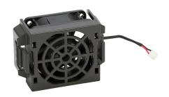
DURApulse GS20 series main cooling fan, replacement,  $60 \times 60 \times 25$ mm, 12 VDC. For use with GS10 and GS20 series D frame AC drives. Electrical connector included.
