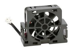
DURApulse GS20 series main cooling fan, replacement,  $40 \times 40 \times 15$ mm, 12 VDC. For use with GS10, GS20 and GS30 series B frame AC drives. Electrical connector included.
