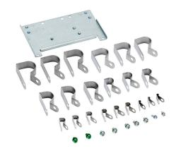
DURApulse GS20 EMC shield plate, for use with GS20 and GS30 series E frame AC drives. Allows motor lead shields to be grounded at the drive.
