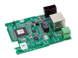
DURApulse GS20 series communication module, EtherNet/IP and Modbus TCP, 1 port, (1) Ethernet (RJ45) port(s). For use with GS20 and GS20X series AC drives.
