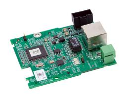
DURApulse GS20 series communication module, EtherNet/IP and Modbus TCP, 1 port, (1) Ethernet (RJ45) port(s). For use with GS20 and GS20X series AC drives.
