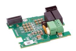
DURApulse GS20 series backup power supply module, for use with GS20 and GS20X series AC drives.
