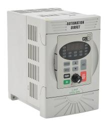
AutomationDirect GS2 series AC micro drive, enclosed, 575 VAC, 1hp with 3-phase input, V/Hz mode, A frame, RS-232/RS-485, integrated dynamic braking.
