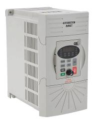
AutomationDirect GS2 series AC micro drive, enclosed, 460 VAC, 7-1/2hp with 3-phase input, V/Hz mode, B frame, RS-232/RS-485, integrated dynamic braking.
