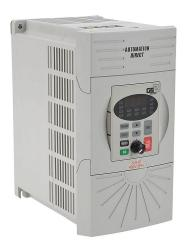
AutomationDirect GS2 series AC micro drive, enclosed, 460 VAC, 5hp with 3-phase input, V/Hz mode, B frame, RS-232/RS-485, integrated dynamic braking.
