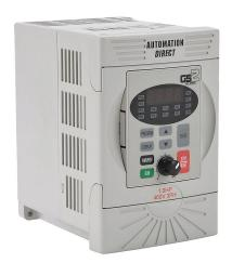
AutomationDirect GS2 series AC micro drive, enclosed, 460 VAC, 1hp with 3-phase input, V/Hz mode, A frame, RS-232/RS-485, integrated dynamic braking.
