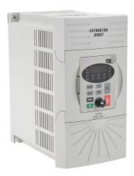
AutomationDirect GS2 series AC micro drive, enclosed, 230 VAC, 5hp with 3-phase input, V/Hz mode, B frame, RS-232/RS-485, integrated dynamic braking.
