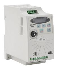
AutomationDirect GS1 series AC micro drive, enclosed, 230 VAC, 1hp with 3-phase and 1-phase input, V/Hz mode, A frame, RS-485, none.
