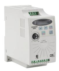
AutomationDirect GS1 series AC micro drive, enclosed, 230 VAC, 1/2hp with 3-phase and 1-phase input, V/Hz mode, A frame, RS-485, none.
