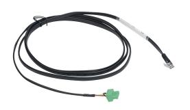
ZIPLink GS drive cable, 6-pin RJ12 to 5-pin terminal block, 6.5ft/2m cable length. For use with GS series drives and FA-ISOCON converter.
