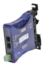
AutomationDirect ethernet communication module, (1) Ethernet 10/100Base-T (RJ45) and (1) RS-232/RS-485 (RJ12) port(s), (12) simultaneous Ethernet connections, (1) serial device(s), 12-48 VDC required. For use with GS1, GS2, GS3 and GS4 series AC drives.
