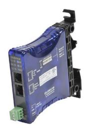
AutomationDirect ethernet communication module, (1) Ethernet 10/100Base-T (RJ45) and (1) RS-232/RS-485 (RJ12) port(s), (12) simultaneous Ethernet connections, (1) serial device(s), 12-48 VDC required. For use with GS1, GS2, GS3 and GS4 series AC drives.
